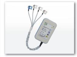
In connection with the MIPM MRI ECG pad the digital artifact filter ensures reliable ECG readings during the full course of a scanning procedure, even during strong gradient scanning sequences.
